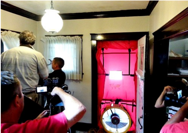
Main entrance to the WV CAG house covered by "blower door" set up to create negative pressure in house to find air leaks.
